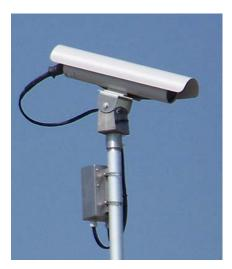
Many municipalities now require video detection for their signal systems. The video cameras are placed on the mast arm assembly as seen in the illustration. This method is often preferable because it is not affected by roadway resurfacing projects that would destroy in pavement loops.
