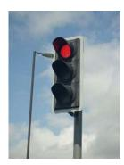
A pedestal (post-mounted) signal may be used in areas with right-of-way constraints or vertical clearance concerns. Due to driver expectancy, span wire or mast arm assemblies are preferred over pedestal assemblies.
